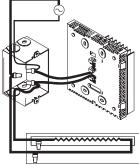
Push any excess wire back into the electrical box.
